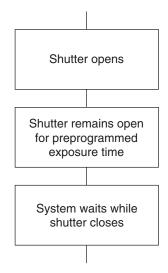
Figure 10. Free Run Timing Chart, part of the chart in Figure 9
